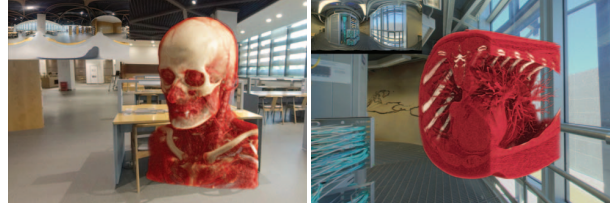
Figure 4: Interactive realistic visualization of medical volume data displayed in our MR prototyping system can respond to the dynamic environment illumination in real time.
