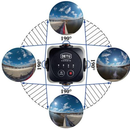
**Figure 1:** Image acquisition using a quad-fisheye camera. Each lens has a FOV of  $190^\circ$  and two adjacent lenses have an overlapping FOV of  $100^\circ$ .
