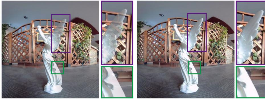
**Figure 15:** Comparison results obtained without (left) and with (right) the inter-lens parallax optimization.
