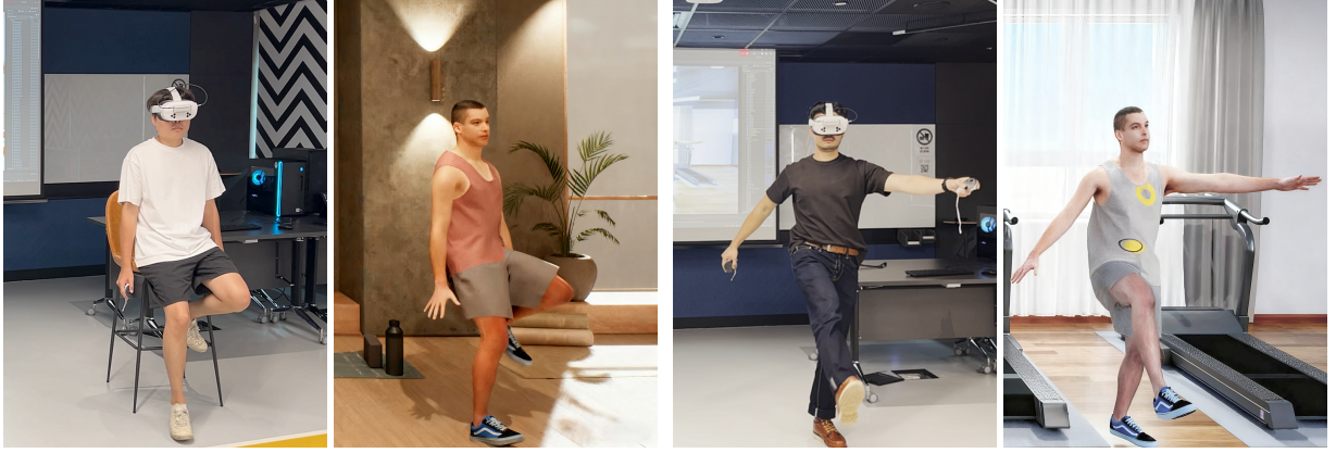
Fig. 1: Egocentric full-body pose estimation in VR enabled by an integrated setup that combines a VR headset with hand controllers and a headset-mounted downward-facing RGB-D camera. The configuration supports real-time and accurate tracking of both upper- and lower-body movements to facilitate natural avatar control and immersive interaction.
